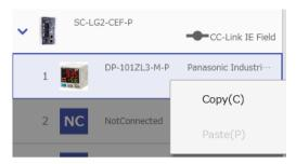
Executing the Copy function causes the frame of the target IO-Link device to blink.
