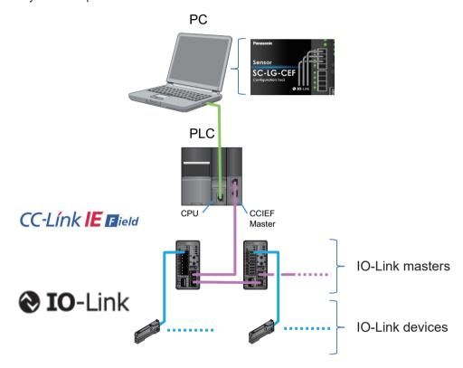
The PC and PLC are connected with an Ethernet or USB cable.
