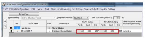
**6.** After setting up the configuration, click the **Close with Reflecting the Setting** menu to close the **CC IE Field Configuration** dialog box.
